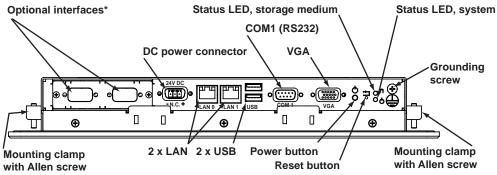
\*Optional interfaces: RS422/485 (insulated), industrial fieldbus, industrial Ethernet...
